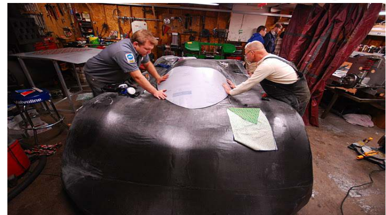
Day 3: Team lays up carbon-fiber composite shell to cure on mold
