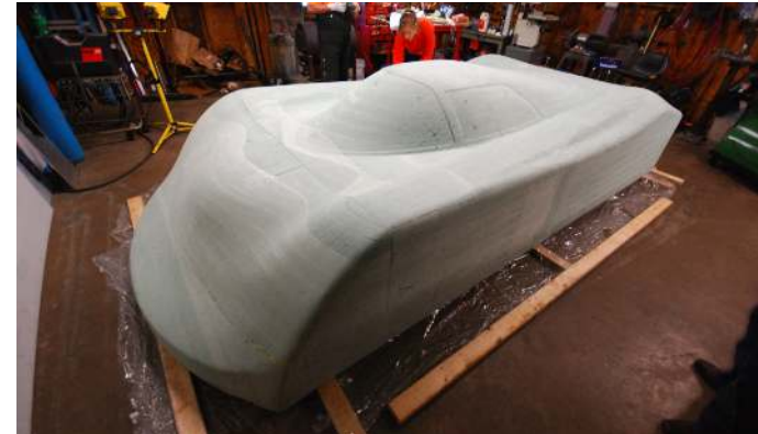
Day 2: Automated CNC router creates foam mold
